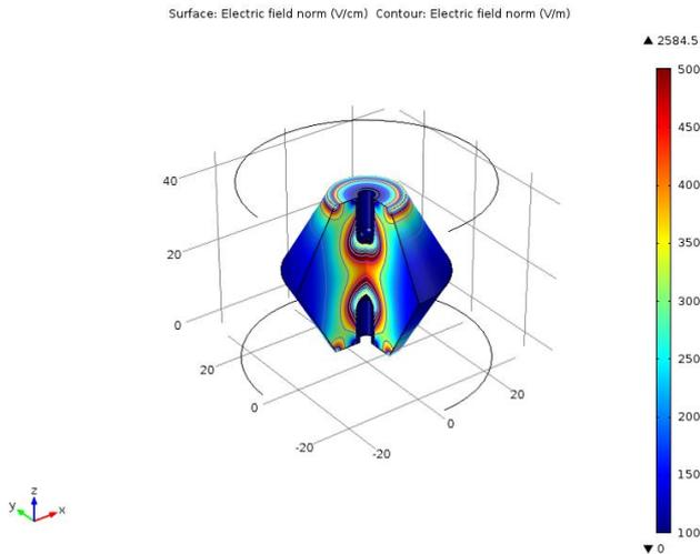
Figure 3. Insulator 3D electrical field simulation
