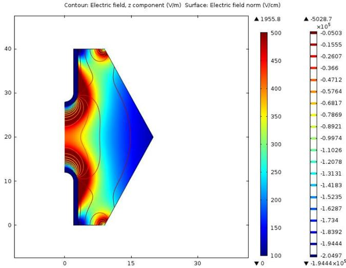
Figure 2. Insulator 2D electrical field simulation
