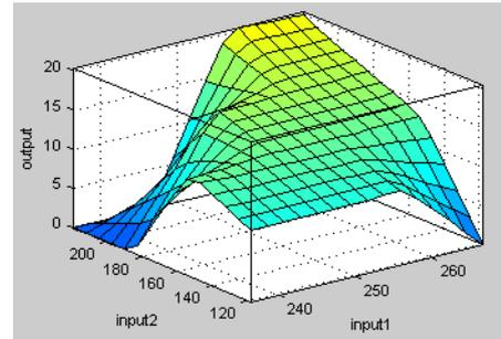
Figure 8. Control surface for a given rule base
