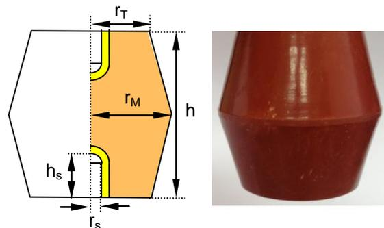
Figure 1. Shuttle insulator
